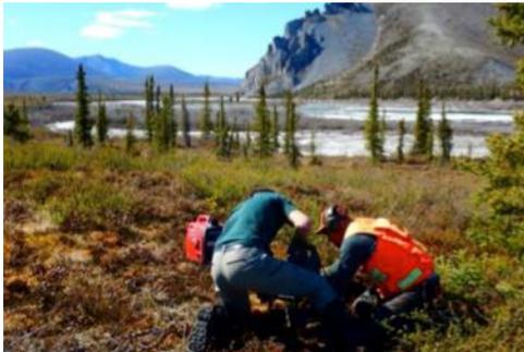
This pilot project uses new innovative sensors called FrostLink sensors to collect active layer temperatures. Twenty-five sensors were installed in four different areas. Terrain at the installation sites was classified to facilitate the interpretation of results.
